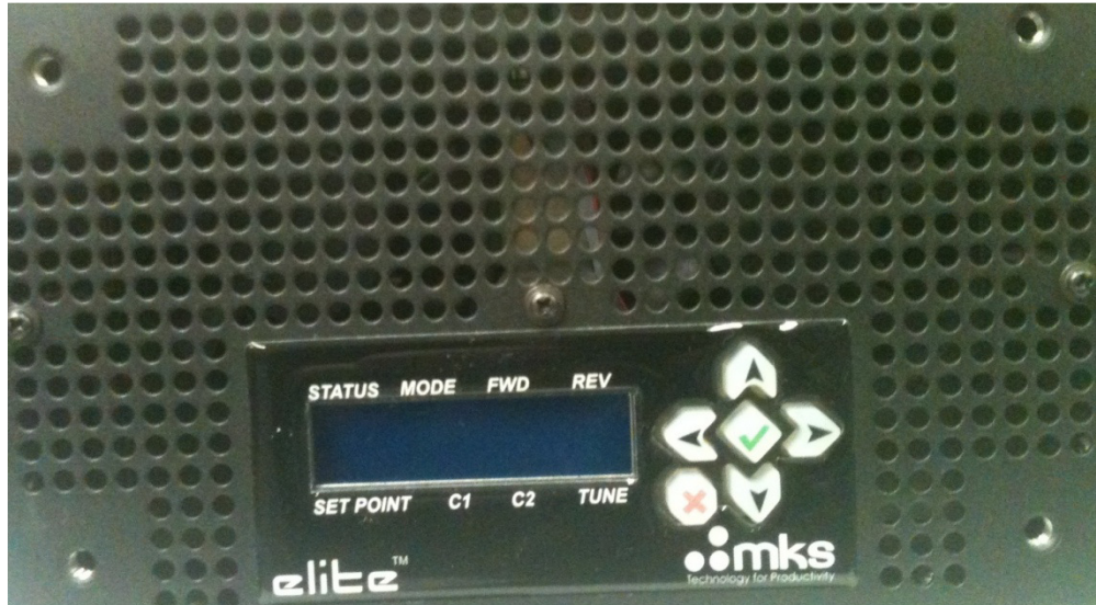
Figure 2-5: RF Generator Supply
